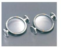
$\pm$  0.37 /  $\pm$  0.50D cross cylinder, + 2.00D retinoscopic lens.
